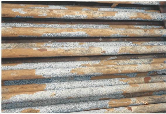
Ammonia tubes much cleaner---- more efficient cooling! Remaining scale on tubes became thinner and falling off in flakes Solenoid valves no longer require frequent scale removal
